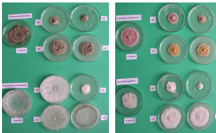
Fig. 1a. Effect of Amistar 250 SC and Biosept 33 SL on the growth of fungi on potato-dextrose agar after 12 days (photo by A. Jamiołkowska): A1 – Amistar concentration 0.05%; A2 – Amistar concentration 0.1%; B1 – Biosept concentration 0.1%, B2 – Biosept concentration 0.2%
