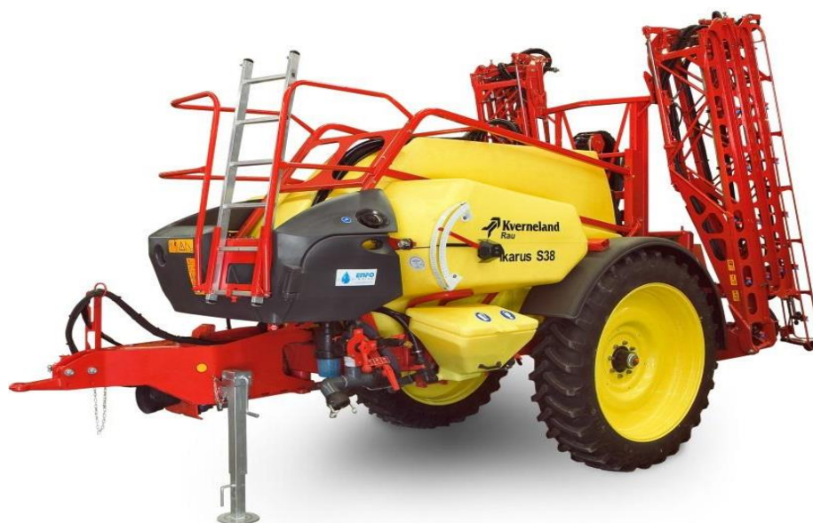
Rys. 4. Przyczepiany opryskiwacz firmy Kverneland [https://pl.kverneland.com] Fig. 4. Trailed field sprayer of Kverneland corporation [https://pl.kverneland.com]
