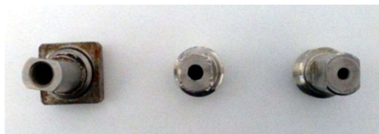
Rys. 4. Głowice prasy ślimakowej o średnicy otworu (od lewej): \varphi_3 = 6 mm, \varphi_2 = 4 mm i \varphi_1 = 2 mm Fig. 4. Heads of a screw press; with the diameter of the hole, respectively: \varphi_3 = 6 mm, \varphi_2 = 4 mm and \varphi_1 = 2 mm
