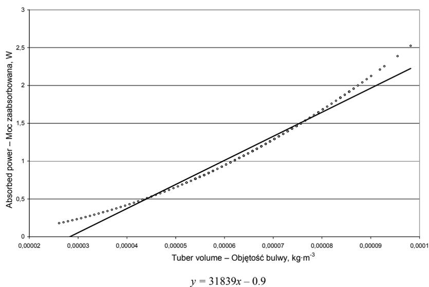
Fig. 2. The relationship between the power absorbed by the microwave-irradiated potato tuber and its volume
