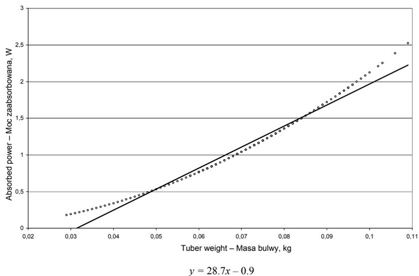
Fig. 1. The relationship between the power absorbed by the microwave-irradiated potato tuber and its weight
