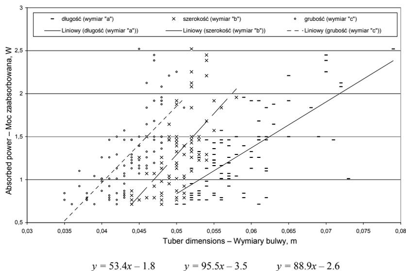
Fig. 3. The relationship between the power absorbed by the microwave-irradiated potato tuber and its dimensions
