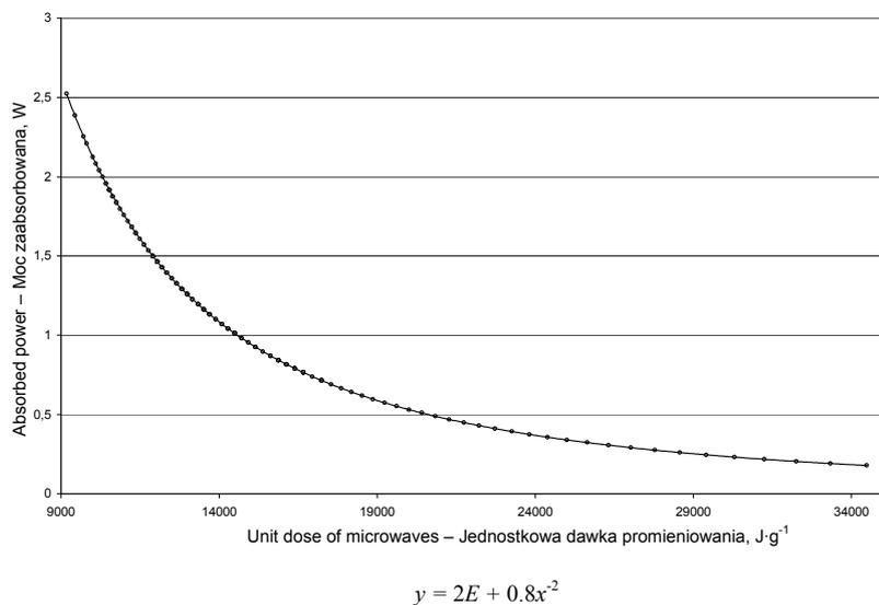
Fig. 4. The relationship between the value of power absorbed by the irradiated potato tuber and the unit dose of microwaves
