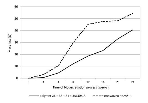
**Fig. 3.** Mass loss in the polymer 26 + 33 + 34 + 35/30/13 granules and nonwoven SB28/13 (AAC made from 26 + 33 + 34 + 35/30/13 with addition of plant biomass) during the biodegradation process (Exp. III)
