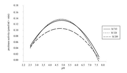
Fig. 2. Effect of pH on the activity of pectinases produced by B. strasseri
