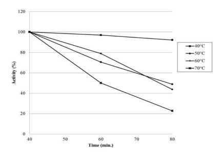
Fig. 6. Thermostability of the pectinases produced by isolate M 743 *B. strasseri* at temperatures ranging from 40 to 70°C
