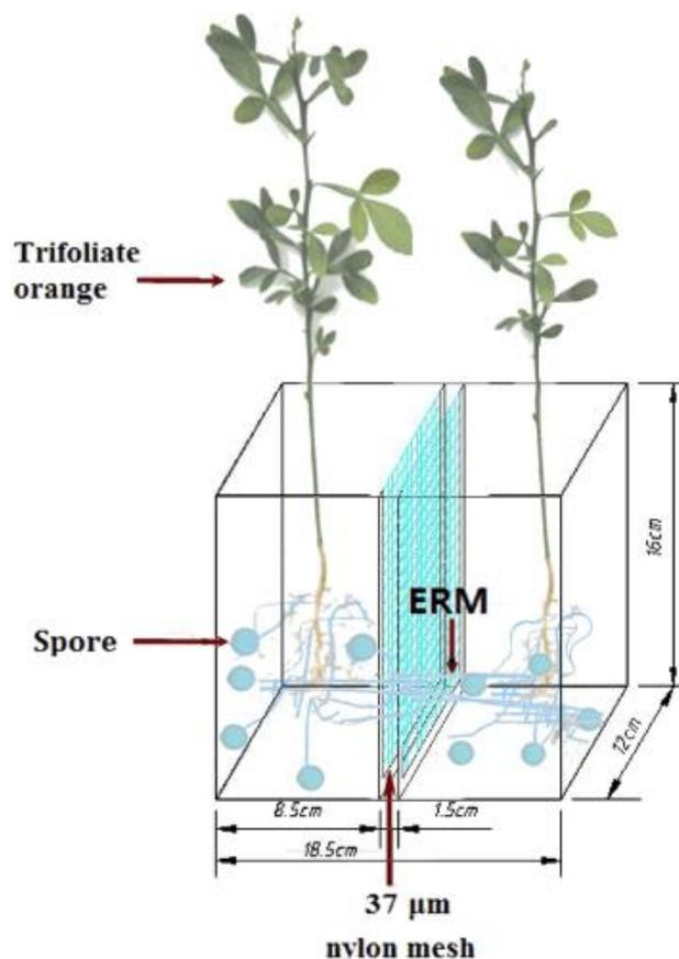
**Fig. 1.** Schematic diagram of the two-chambered rootbox. Here, mycorrhizal donor plants with *Paraglomus occultum* developed extraradical mycelium (ERM), which can pass through 37 µm nylon mesh into receptor chamber to colonize receiver plants
